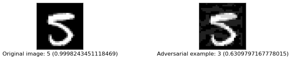
Figure 1.1: Adversarial example on the MNIST dataset. Number in brackets is confidence of the network
