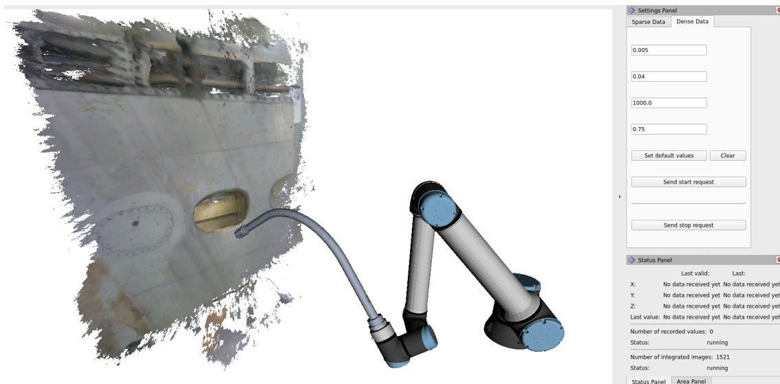
Figure 2.9: Eeloscope2 on UR10e arm inspecting an aircraft wing [Ric24]
