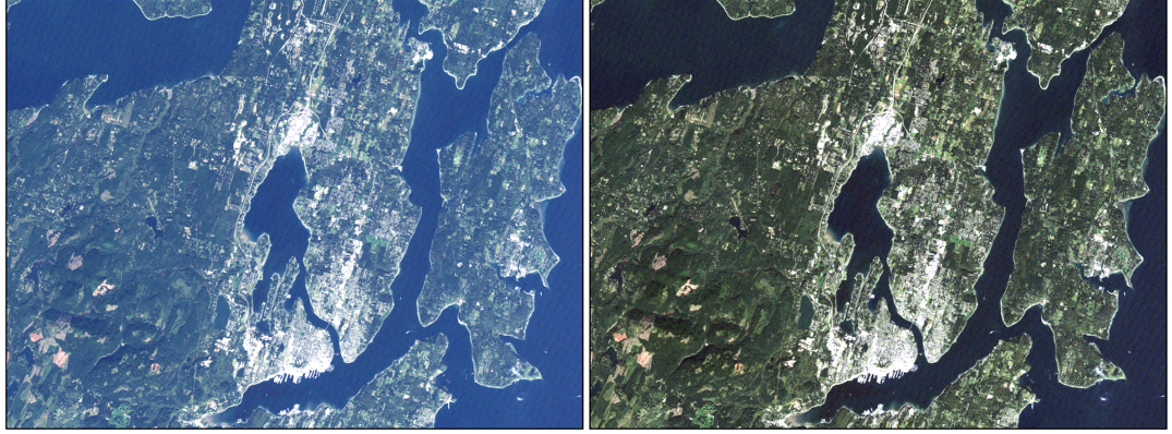
Figure 2.1: Inversion example showing TOA (left) and surface reflectance (right). Image taken from USGS [6].
