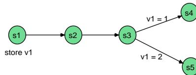
**Fig. 4.** Data dependent routing
