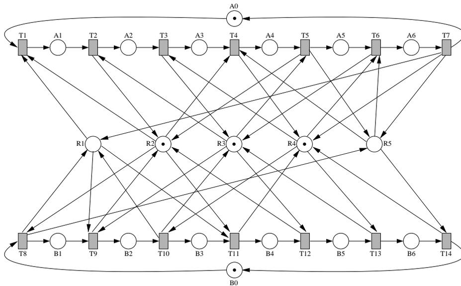
Fig. 7. A marked SB SPQR which is live but has no home states
