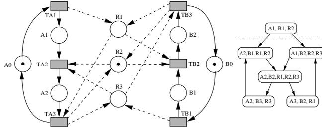
Fig. 6. An acceptably marked PC<sup>2</sup>R which is live but not reversible
