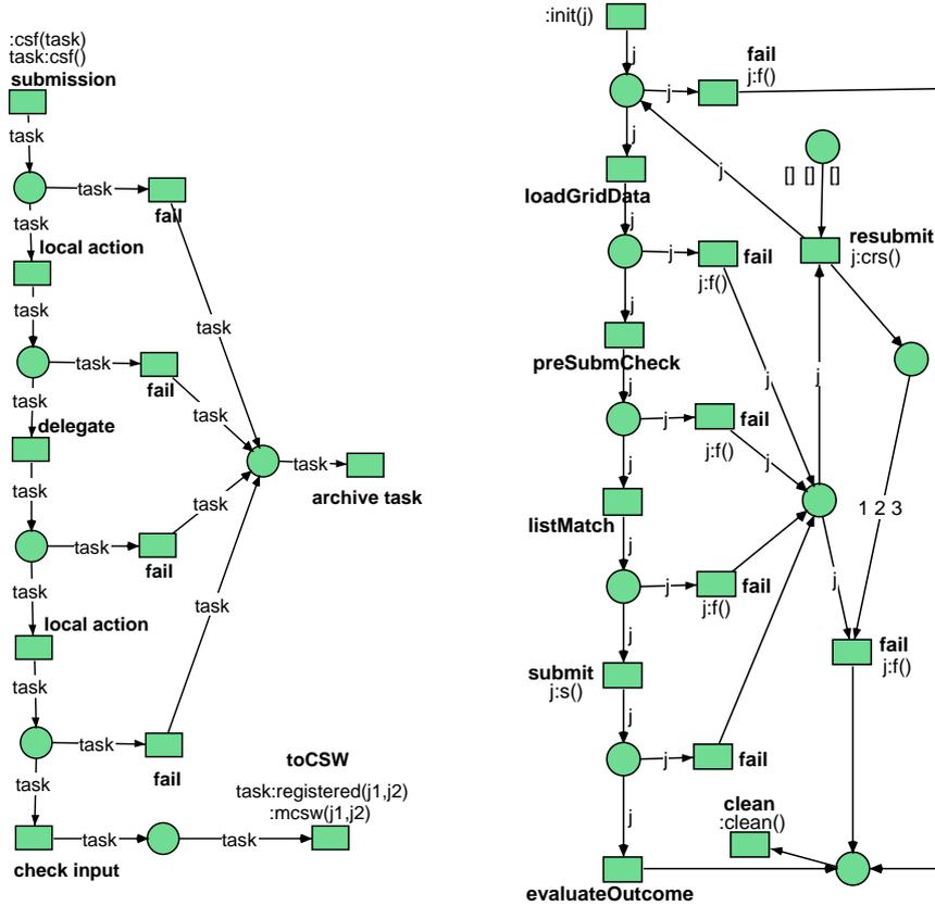
Fig. 7. TaskRegister and SubmissionWorker nets respectively
