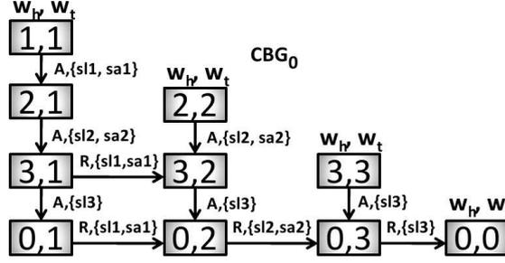
Fig. 4. Conveyor Behaviour Graph for destination workstation 0.
