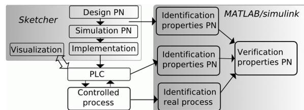
Fig. 1. Verification hybrid Petri nets
