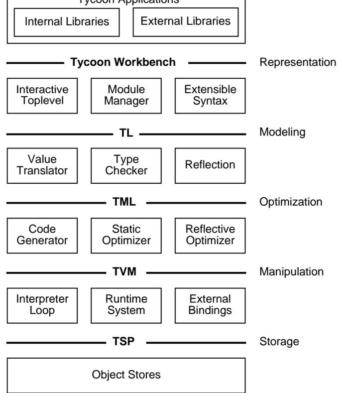
Fig. 4. Layered Architecture of the Tycoon System
