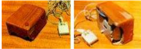
Fig. 3.3 The first wooden mouse, invented by Doug Engelbart and Bill English at SRI in 1963
